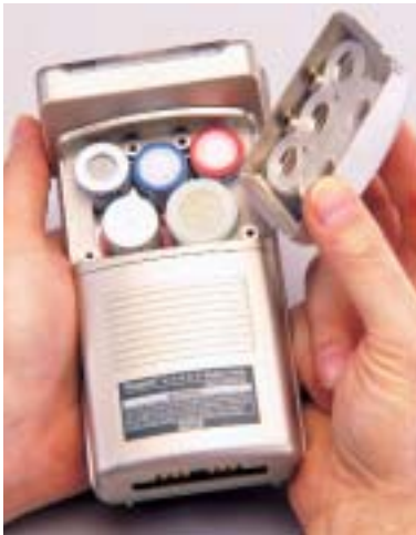
Choose up to five different sensors to configure the FiveStar for your need.
