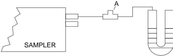
2. On the open end of the "T," draw vacuum by mouth until 4 to 5 inches of water vacuum register on the manometer.
